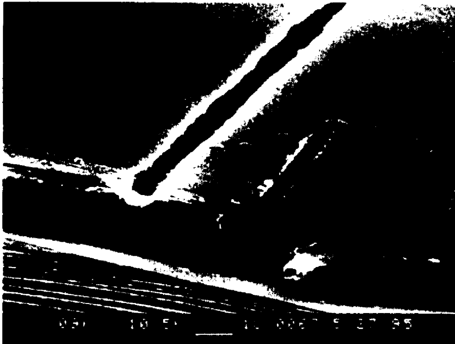
Figure 6.5. A micrograph showing problems related to improper mounting of the sample on the sample holder.
